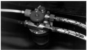
For pure single-pipe operation the bypass stopper must be unscrewed out of the return line opening (2) and the return line opening must be sealed with a gasket and metal stopper.
